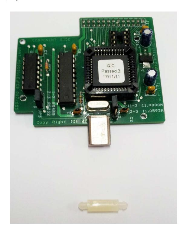
3.) Plug stand into the UART Board at the red point follows picture below.
